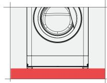
The washing machine should always be installed on a flat solid surface free from sloping, unevenness or any flexing.
