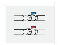
Connect the straight end of the inlet hoses to the appropriate water supply isolating valve. When complete, open isolating valves to let water into the machine.
