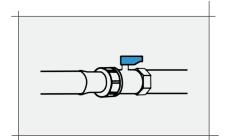
Connect the straight end of the inlet hose to the cold water supply isolating valve. When complete, open isolating valve to let water into the machine.
