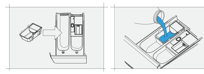
Insert and fix the liquid boat accessory into the main wash detergent compartment.
