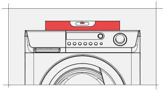
4. Check the washing machine is level and stable using a spirit level. Ensure you adjust the feet so the machine doesn't rock corner to corner.
