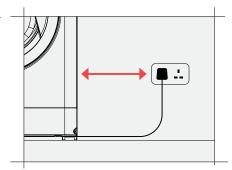
A power supply socket must be within 1.5 metres of either side of the washing machine. Do not overload the socket with multiple appliances.
