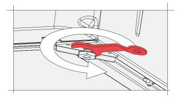
1. Lift the machine up off the floor to access the front feet and loosen the locking nut using the spanner provided.
