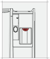
**Softener** Allows liquid softener to be used only. Do not fill above the max indicator line.
