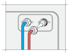
Check the end of each inlet hose to ensure the black rubber seal is fitted. Connect the L-shaped inlet hose ends to the back of the machine.
