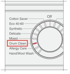
Turn the machine on by turning the dial to select the **drum clean** wash programme. Cotton Sa Eco 40-60 Synthetic-Delicate-Mixed-Drum Clea Allergy Ca Hand/Woo
