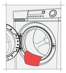
1. Open the door and wipe the door seal using a damp cloth. Before closing the door, ensure the drum is empty.
