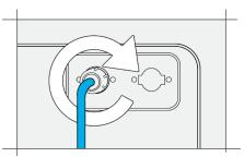
Tighten by hand by turning clockwise. Ensure the hose is not twisted or kinked before connecting the other straight end of the hose.
