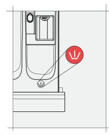
**Prewash** Compartment allows both powder and liquid detergent to be dispensed.
