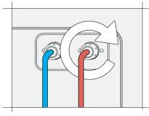
Tighten by hand by turning clockwise. Ensure the hoses are not twisted or kinked before connecting the other straight end of the hoses.
