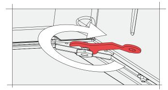
3. Ensure you re-tighten the locking nut to secure the foot into position.
