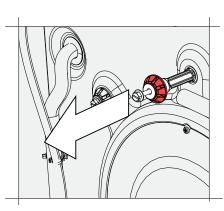
2. Ease out and remove the transit bolt assembly by twisting and pulling on the section highlighted in red on the diagram.
