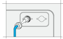
1. Check each end of the inlet hose to ensure the black rubber seal is fitted. Connect the L-shaped inlet hose end to the back of the machine.
