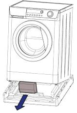
Ensure packaging block is removed with base.
