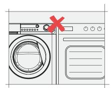
Avoid positioning the washing machine directly next to any gas supplies or appliances such as cookers/hobs.
