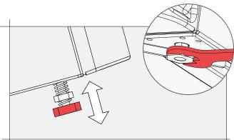
**2.** Adjust to the desired height by turning the foot clockwise / anticlockwise.
