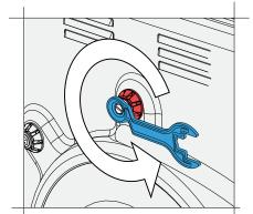
Using a 10mm spanner (supplied), loosen the transit bolt assembly by 25mm.
